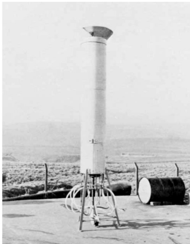
Fig. 8. View of 5 ton/hr low noise flare system.
